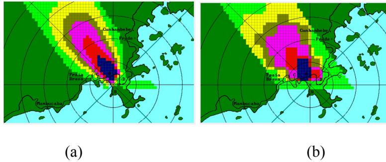
**Figure 6 - Comparisons between (a) simulator; (b) MLP predictions and (c) GRNN predictions for spatial dose rate distribution 1h after an occurring the accident, considering wind velocity=2.5 m/s and wind direction=34°.**
