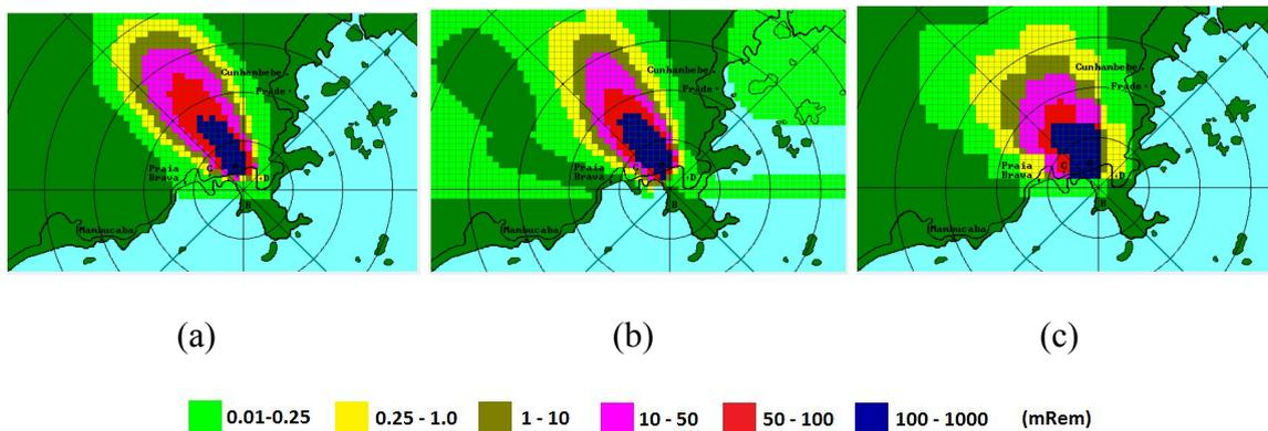
Figure 6 - Comparisons between (a) simulator; (b) MLP predictions and (c) GRNN predictions for spatial dose rate distribution 1h after a occurring the accident, considering wind velocity=2.5 m/s and wind direction=34°.
