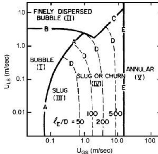
**Figure 4 – Traditional two-phase flow regime map of Taitel et al, for air-water at 25 ° C and 0.1 Mpa in a 50-mm diameter tube.**
